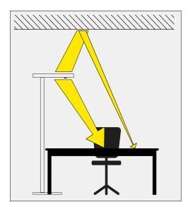
The luminous intensity emitted by a light source decreases proportionally to the covered distance at a factor of x<sup>2</sup>. The ceiling's degree of reflection influences how much light is transferred onto the work surface from the indirect lighting.
